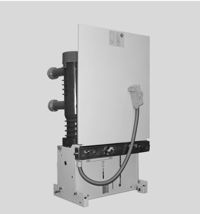
Figure 3/7: Vacuum circuit-breaker, type VD4, with assembled poles and forced ventilation (fan), on withdrawable part, operating mechanism side 2500 A at 55 °C 3150 A, 25/31.5 kA at 40 °C
