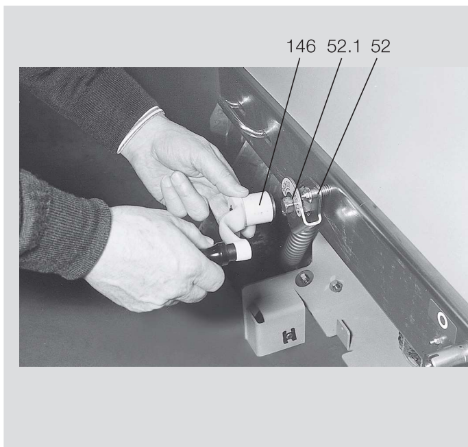
Figure 6/5: Fitting the hand crank (against a spring-loaded plate) – clockwise into the service position – anti-clockwise from the service position into the test/disconnected position
